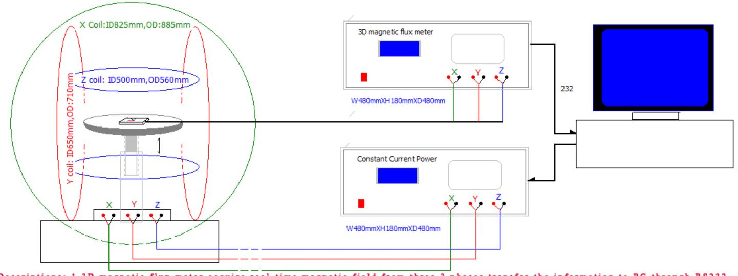
Descriptions: 1.3D magnetic flux meter acquire real-time magnetic field from three 3 phases, transfer the information to PC through RS232.
